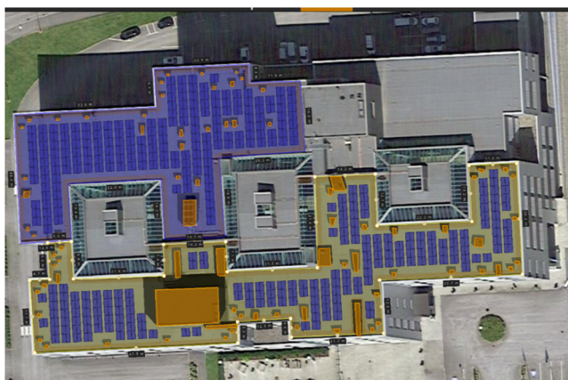
Figure 3. Example of rooftop with marked roof area in blue, solar panels, and excluded roof structure in orange.
