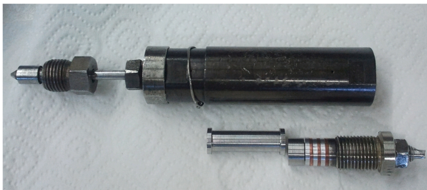
Fig. 2. Zero matrix high pressure TiZr cell with thin stainless steel liner.
