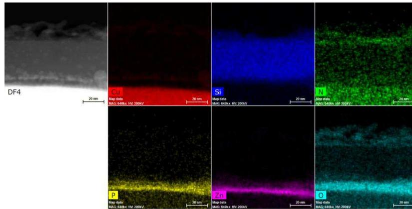
Figure 1: Dark field STEM image and EDS maps of sample E, showing high concentrations of P, Zn and O in the interface between the copper substrate and silicon film.
