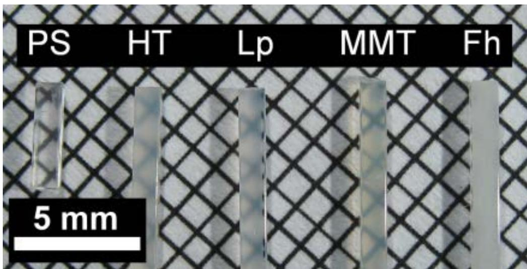
**Figure S1.** Picture of the finished nanocomposites. From left: pure PS, PS-Hectorite (HT), PS-Laponite (Lp), PS-Montmorillonite (MMT) and PS-Fluorohectorite (Fh).
