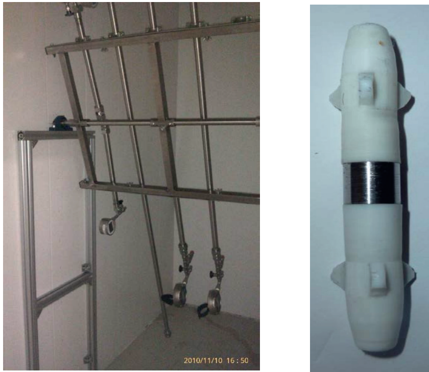
Figure 1. Left: Slim autoclaves rotated in a thermal cabinet. Right: Carbon steel specimens (OD 10 mm, length 10mm) mounted in a 8-10 cm long sliding specimen rack.
