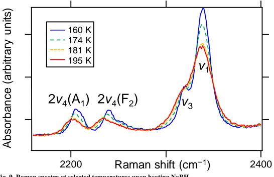
Fig. 9. Raman spectra at selected temperatures upon heating NaBH<sub>4</sub>.
