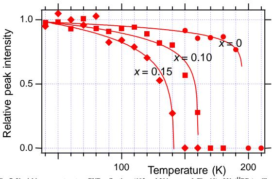
Fig. 7. Vanishing superstructure PND reflections (102 and 201 summed, Fig. 10) of  $Na(^{11}BD_4)_{1-x}Cl_x$  upon heating. The intensities are normalized to the values found at 8 K.
