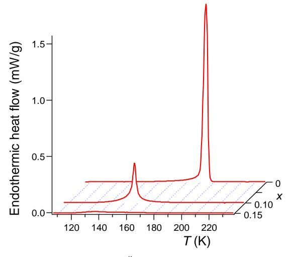
Fig. 2. Endothermic effect upon heating  $Na(^{11}BD_4)_{1-x}Cl_x$  through the order–disorder transition.
