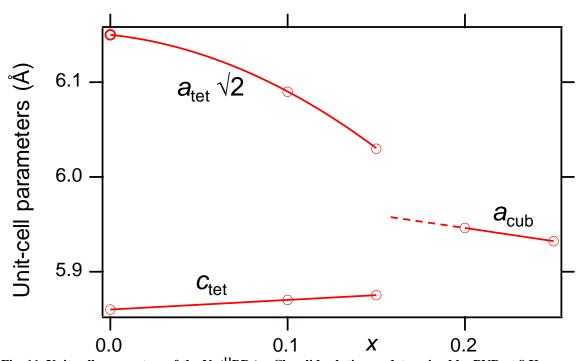
Fig. 11. Unit-cell parameters of the Na(<sup>11</sup>BD<sub>4</sub>)<sub>1-x</sub>Cl<sub>x</sub> solid solution as determined by PND at 8 K. The gradual approach, even at 8 K, of the tetragonal order of the borohydride anions towards the cubic disorder upon increasing frustration by the spectator anion of the solute
