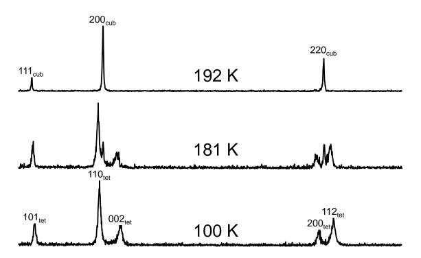
Fig. 8. Comparison of SR-PXD patterns (8 to  $14.5^{\circ} 2\theta$ ) upon heating NaBH<sub>4</sub> of the tetragonal (bottom) and cubic (top) phases, with a range of coexistence (middle) at the transition between 180 and 190 K.
