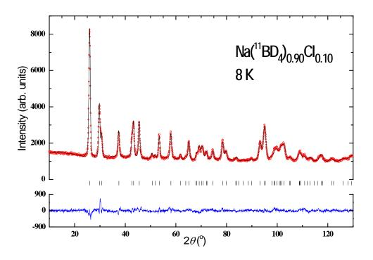
Fig. 12 Rietveld fit showing experimental (black solid line) and calculated (red circles) PND profile of Na(<sup>11</sup>BD<sub>4</sub>)<sub>0.90</sub>Cl<sub>0.10</sub> at 8 K. The blue line is the difference plot. Bragg peaks are marked with vertical ticks;  $R_{F2} = 0.0619$ ;  $\lambda = 1.5556$  Å.
