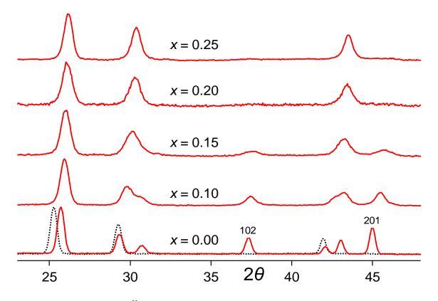
Fig. 10. PND patterns of  $Na({}^{11}BD_4)_{1-x}Cl_x$  at 8 K. Increasing concentration x of the NaCl solute frustrates ordering in the  $Na{}^{11}BD_4$  solvent, as apparent from decreasing intensity of ordered-structure peaks 201 and 102 identified on the x = 0.00 plot, where also the room-temperature pattern is shown for comparison with a dashed line.
