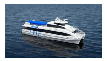
Fig. 2. Illustration of a concept design (GKP7H2) of a hydrogen and fuel cell driven high speed passenger ferry [20].
