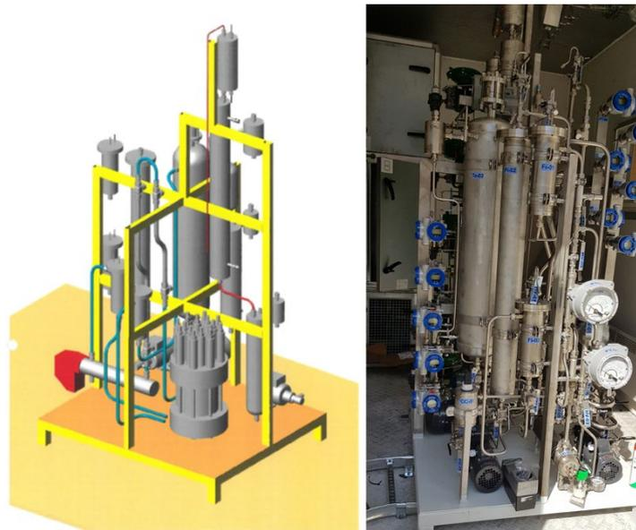
**Figure 2:** Mechanical design and photo of the PEMWE system test rig.
