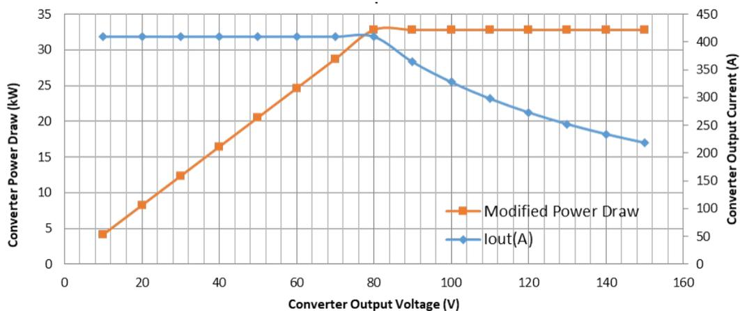
**Figure 4:** Output characteristics of DC/DC converter for water electrolyser system.
