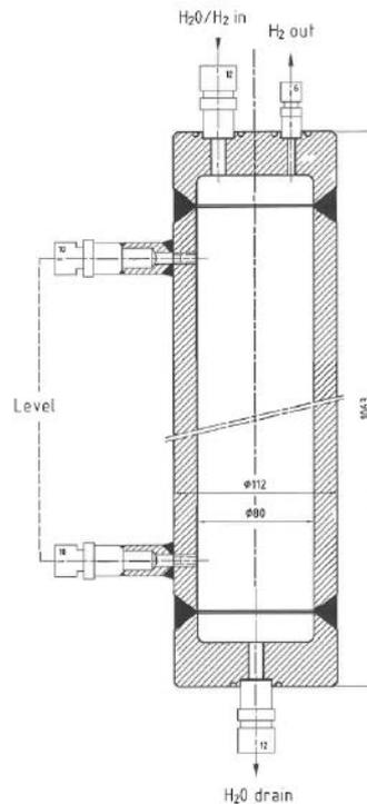
**Figure 7:** Water/hydrogen separator vessel (Ta-03), designed for pressures up to 350 bar.
