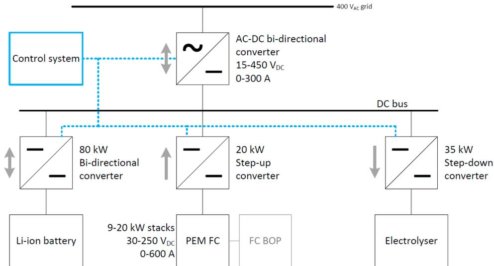
**Figure 3:** Electrical system and power converters of the systems laboratory at IFE.
