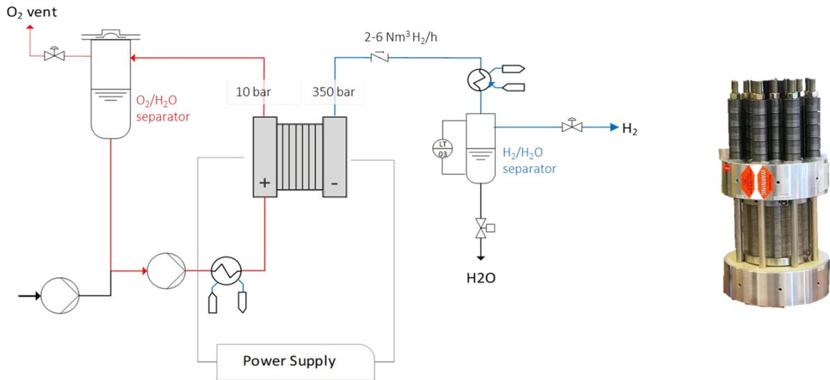
**Figure 1:** Sketch of WE system test rig (left) and prototype PEMWE stack operable at differential pressures up to 350 bar (right).
