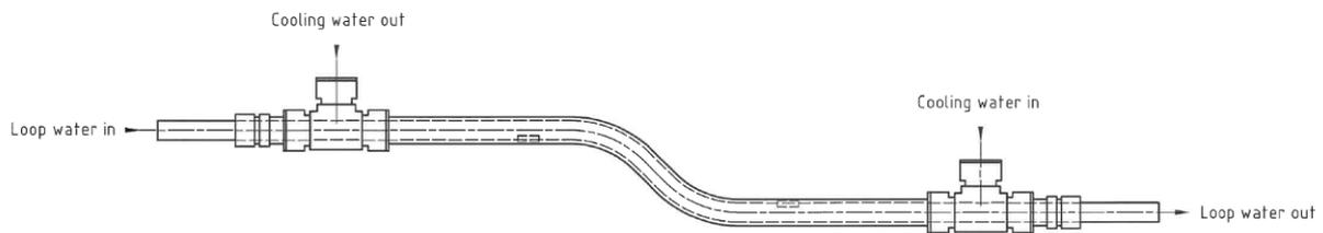
**Figure 6:** Heat exchanger design for E-01 and E-02.
