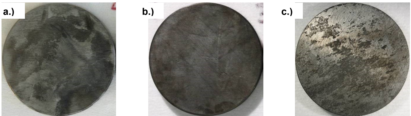
Figure 3: Pictures of carbon steel coupons after exposure at (a) 25 °C, (b) 60 °C and (c) 80°C after stripping in HCl
