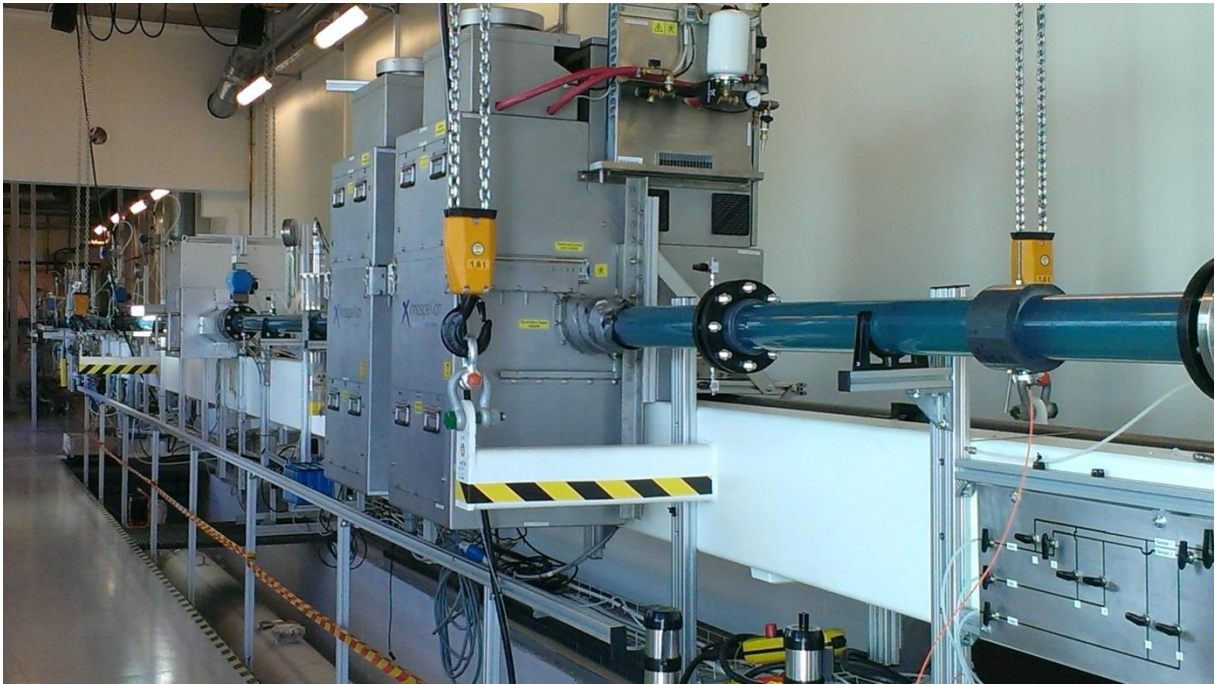
Figure 29: Picture of the Well Flow Loop taken at the near end of the test section, equipped with X-ray tomography systems
