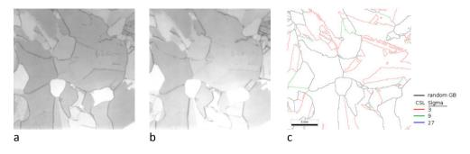
Fig. 8. High magification PL-image of an un-passivated a) ungettered and b) gettered wafer from the upper section of the cast (100% of wafered block height). EBSD map from same wafer position is shown in c).
