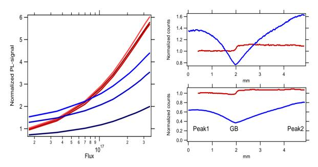
Fig. 9. (a) Normalized PL-signal (against Peak1 ungettered) vs illumination flux for Peak1, GB and Peak2. red) ungettered and blue) PDG. b) Linescans across a the grain boundary b) 1.7e16 and c) 2.1e17 Photons/cm2
