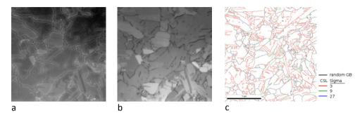
Fig. 3. High magification PL-image of an unpassivated a) ungettered and b) gettered wafer from the bottom section of the cast (4% of ingot height). EBSD map from same wafer position is shown in c).
