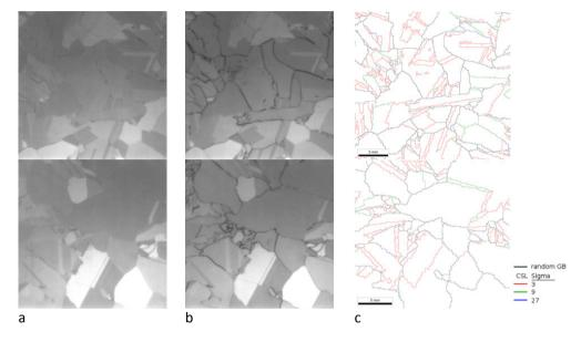
Fig. 5. High magification PL-image of unpassivated a) ungettered and b) gettered wafer from the middle section of the cast (Upper row 30% and lower row 60% of ingot height). EBSD map from same ingot height is shown in c).
