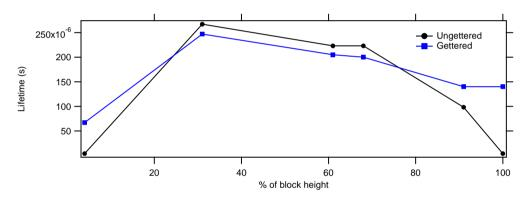
Fig. 2. QSSPC lifetime at 1e15 cm-3 (or maximum injection level) as a function of height in the block.
