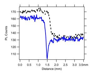
Fig. 6.PL signal at a RA grain boundary. Dashed line show ungettered and solid line is after PDG.
