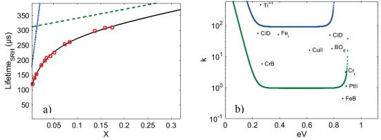
**FIGURE 3.** a) Linear parameterization of the lifetime before gettering showing a two defect fit. b) DPSS for two dominating recombination centers corresponding to the parameterization in a).
