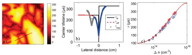
FIGURE 2. a) PL-image of 2x2 cm area, the line indicates where the carrier profile has been measured b) grey - measured steady state carrier profile, blue - carrier profile used for simulations of recombination profile and black - the fitted recombination profile. c) Injection dependent lifetime curve, blue circles – from raw data and red squares – simulated bulk lifetime. The solid red line corresponds to two defect fit of the lifetime according to the solution in Fig. 3.
