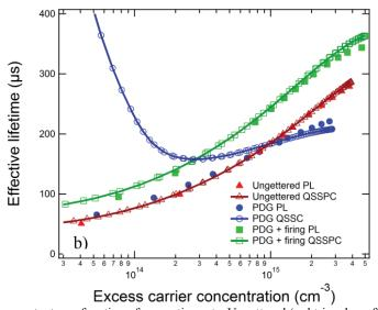
FIGURE 1. a) Calibration constant as a function of generation rate. Ungettered (red triangles, after PDG (blue dots) and after PDG and fired (green squares). The lines are a guide to the eye. b) Effective lifetime vs. excess carrier concentration after three different stages of solar cell processing. The filled symbols are from PL-images, whereas open symbols + lines are from QSSPC measurements.
