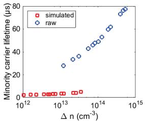
FIGURE 4. Lifetime measured at GB in steady state PL-image (blue circles) and – lifetime corrected for transport of carriers according to simulated recombination profile (red squares).
