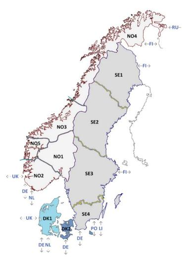
Figure 1: Illustration of the Scandinavian Nord Pool price areas, with indication of existing and proposed transmission capacities to surrounding countries; Finland (FI), Poland (PO), Lithuania (LI), Germany (DE), the Netherlands (NL) and the United Kingdom (UK).
