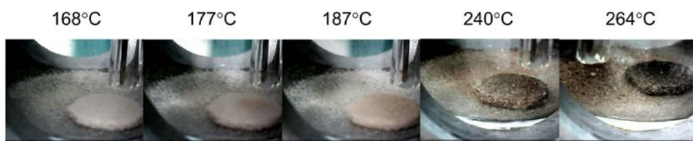
Fig. A2 TPPA pictures showing the white pellet consisting of \text{Er}(\text{BH}_4)_4 + \text{KBH}_4 (168 °C; far left), the onset of \text{KEr}(\text{BH}_4)_4 formation seen as a pink spot (177 °C), the pink color of the pellet after full conversion to \text{KEr}(\text{BH}_4)_4 (187 °C) and the dark pellet during different stages of the decomposition (240 °C and 264 °C). No melting is observed at any temperature up to 500 °C.
