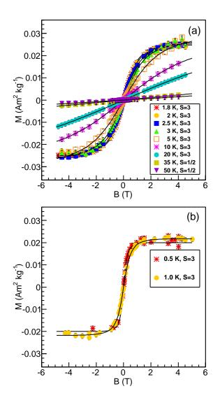
Figure 4: (Color online) Magnetization M vs magnetic field B at selected temperatures in the intervals (a)  $1.8 \leq T < 50$  K and (b) T = 0.5 and 1 K. Here, the magnetization of the gelatin capsule, the ferromagnetic background of metallic impurities and the diamagnetic background of the carbon powder have been subtracted from the measured data. Solid lines show approximations to these corrected data based on Eq. 2. For each temperature, the value of S that gave the best fit is shown.
