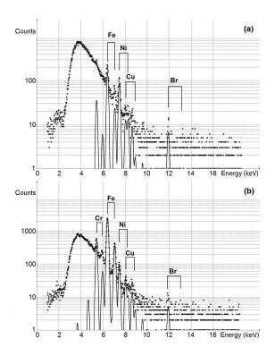
Figure 1: PIXE spectra of (a) the pure Cyclopore Membrane and (b) typical PIXE spectra of HT-1600 carbon powder on a Cyclopore Membrane.
