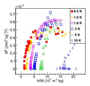
Figure 6: (Color online) Arrott plots of the background corrected data in the temperature range  $0.5 \le T \le 10$  K.
