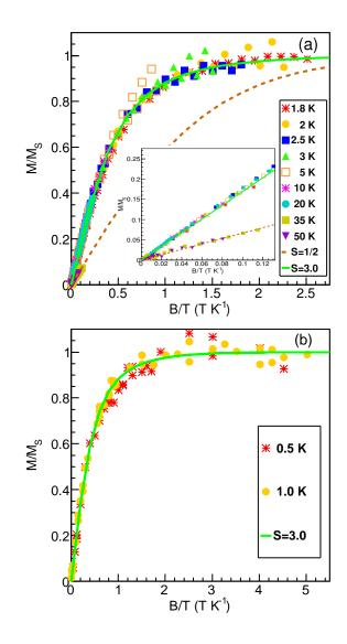
Figure 5: (Color online)  $M/M_S$  vs B/T plots for temperatures (a)  $1.8 \le T \le 50$  K and (b) T = 0.5and 1 K. Solid lines show approximations to these corrected data based on Eq. 2 using either S = 1/2 or S = 3. The inset shows a detail near origin of coordinate axes.
