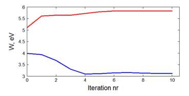
**Figure 6.** Convergence of quasiparticle energies in the self-consistent GW calculations. The upper red line corresponds to the bottom of the conduction band; the lower blue line corresponds to the top of the valence band.
