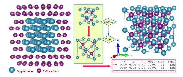
**Figure 1.** Flowchart illustrating a copper-driven assembly of  $\gamma$ -CuI in the Cu-I system. Metallic copper represents a crystalline bulk template in which the packing of iodine atoms proceeds through the filling of interstices. Structural relationship between the template and the final phase is determined by the group-subgroup relation  $Fm\bar{3}m \rightarrow F\bar{4}3m$ .
