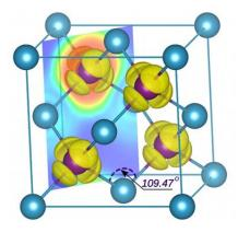
**Figure 4.** Visualization of the valence electron density of CuI pictorially represented by the ELF isosurface at ELF=0.86. The covalent bonding is associated with the regions of localized electron pairs. The shift of the electron clouds towards iodine reflects the polar character of the shared electron connections. 109.47 ° is the bond angle in a tetrahedral environment.
