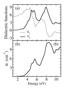
**Figure 7.** Many-body simulation of optical responses of  $\gamma$ -CuI. **A.** Real and imaginary parts of the frequency-dependent dielectric function. **B.** Absorption spectra.
