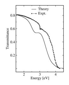
*Figure 8.* Transmission spectra for  $\gamma$ -CuI calculated by self-consistent GW calculations in this work (—) as compared to that measured experimentally in Ref.[14] (•—•).
