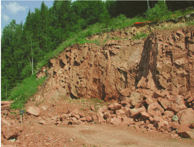
Figure 4 - The Brumunddal sandstone at the quarry close to the Mauset school. The picture gives a general impression of the relatively homogeneous red sandstone, the bedding and the fracture system.
