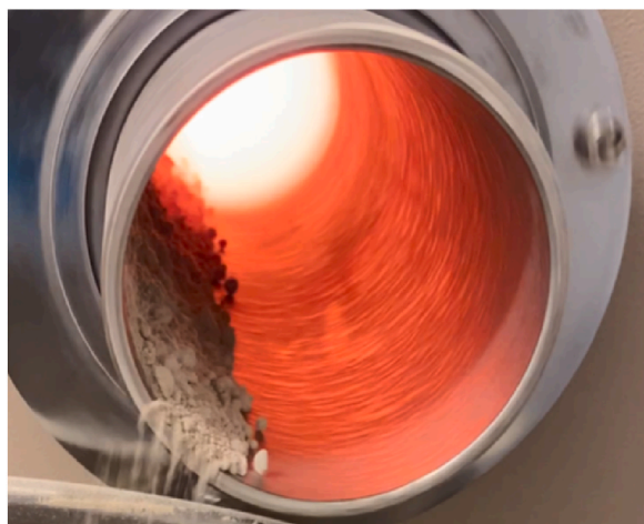
Fig. 3. Outflow of agglomerated particles from the rotary calciner.
