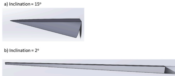
Fig. B2. Geometrical view of 200 g of particles inside the calciner inclined at a) 15° and b) 2°.
