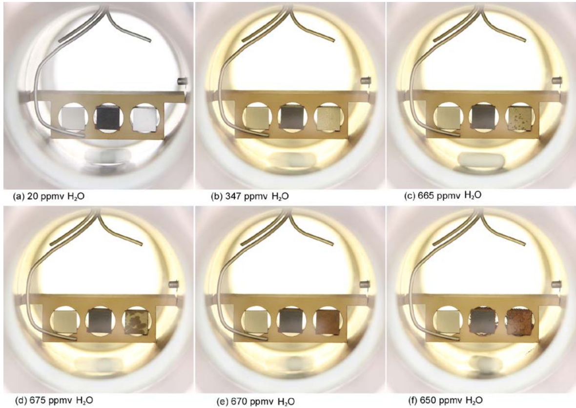
FIGURE 10. Still pictures from Exp-04. The left, center, and right-hand side corrosion coupons were, respectively, duplex stainless steel, carbon steel with mill scale, and polished carbon steel.
