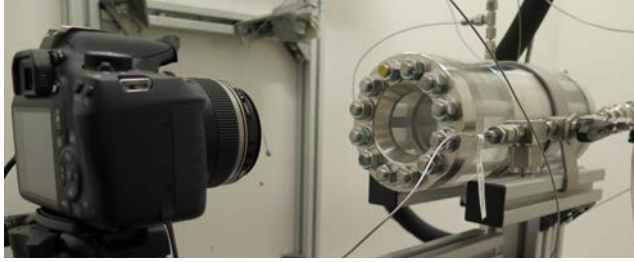
FIGURE 1. Photo showing the transparent autoclave with camera and injection tubing.
