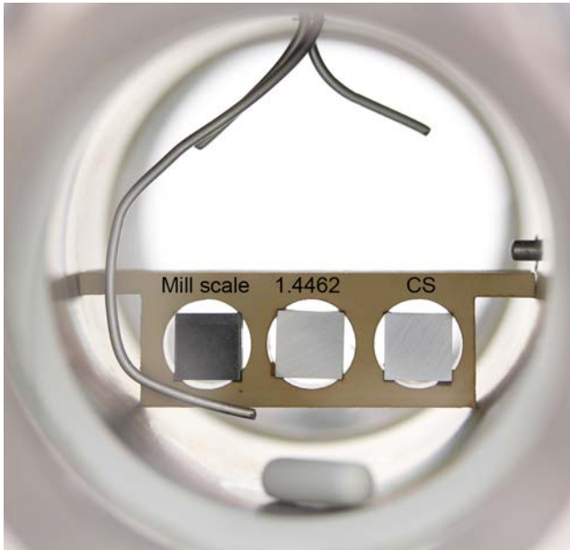
FIGURE 2. Photo of the autoclave interior with coupon holder and three coupons and the stirring magnet. The impurities were injected through the tubes from the top.
