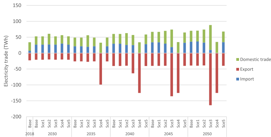
Fig. 5. International and domestic electricity trade in Norway until 2050. Sce1 = transmission lines, international; Sce2 = transmission lines, domestic; Sce3 = offshore wind, Sce4 = onshore wind, Sce5 = solar PV.
