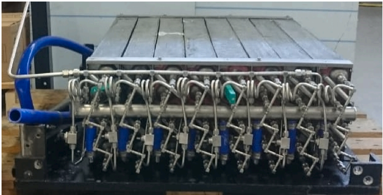
Fig. 8. HySA Systems tank made as an assembly of lead-encased MH cassettes for hydrogen storage on-board of fuel cell forklift [227].
