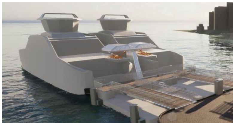
Figure 5: Fully automatic pantograph delivered by SEAM
