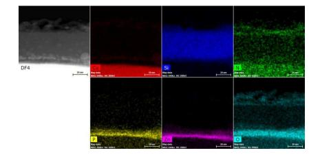
Figure 1: Dark field STEM image and EDS maps of sample E, showing high concentrations of P, Zn and O in the interface between the cupper substrate and silicon film.
