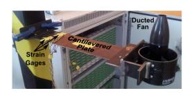
Figure 5. Fan Set Up for Calibration
