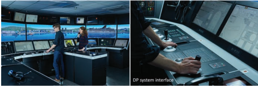
FIGURE 15.1 Modern ship bridge environment with dynamic positioning (DP) systems. (Training simulator, photo by Kongsberg Maritime.)
