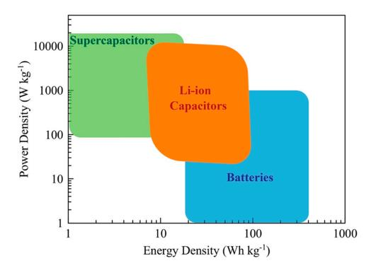
**Figure 1.** Qualitative Ragone plot reported in normalized terms of mass of the whole device. The shaded areas are reported in gravimetric terms.
