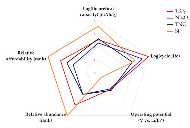
**Figure 9.** A "spider web" or "radar" chart can comparatively evaluate the complex performance-determining parameters of different materials with greater detail than a Ragone plot. Cycle life and theoretical capacity are plotted on a log scale for clarity. For ranked parameters, higher values indicate higher rank (e.g., Si is relatively the most abundant material of the four selected here).
