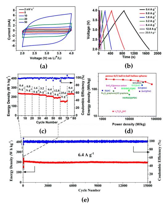
**Figure 5.** Performance of porous Si/C ball-in-ball HSs: (**a**) CV curves at different scan rates; (**b**) voltage profile; (**c**) rate performance; (**d**) Ragone plot, and (**e**) long cycling performance at 6.4 A  $g^{-1}$  of a Si@C ball-in-ball HSs||RAC LIC full cell. Adapted from [89].
