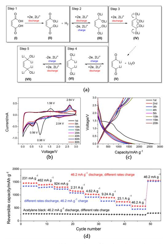
**Figure 8.** (a) Structure & proposed lithiation mechanism of the maleic acid as an anode; (b) cyclic voltammograms and (c) voltage profiles and charge and discharge profiles at 46.2 mA g<sup>-1</sup> in the voltage range of 0.01–3.0 V; (d) rate capability at room temperature (red and blue line correspond to charge and discharge, respectively). Adapted from [110].
