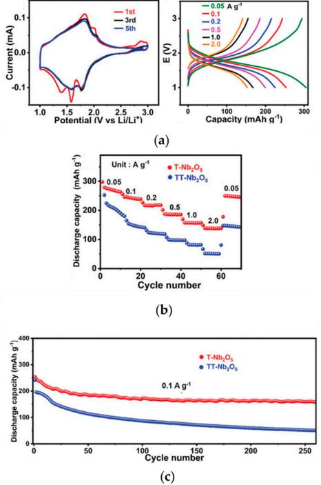
**Figure 3.** (a) Cycling Voltammetry (CV) curves  $(0.1 \text{ mV s}^{-1})$  (left panel) and galvanostatic chargedischarge plots at various current densities of T-Nb<sub>2</sub>O<sub>5</sub> nanorods (NRs, right panel); (b) rate behaviors of T-Nb<sub>2</sub>O<sub>5</sub>; (c) Cycling properties of T-Nb<sub>2</sub>O<sub>5</sub> and TT-Nb<sub>2</sub>O<sub>5</sub> NRs at 0.1 A g<sup>-1</sup>. Adapted from [52].
