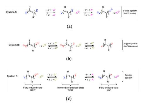
**Figure 6.** (**a**–**c**) 3 general key redox-active organic systems and their related charge transfer steps (adapted from Hünig's classification [104]).
