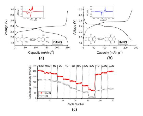
**Figure 7.** (**a**,**b**) show two-electron electrochemical lithiation and delithiation of 2,3-diamino-1,4naphthoquinone (DANQ) and 1H-naphtho [2,3-d]imidazole-4,9-dione (IMNQ), respectively; (**c**) rate performance of the Li-DANQ cell compared to Li-NQ cell. Adapted from [108].
