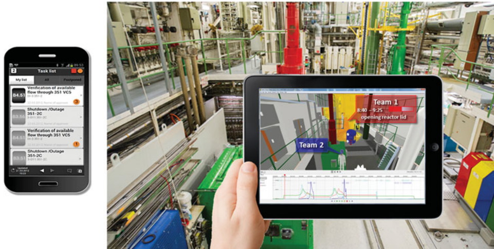
Figure 11. In situ information for field operators showing task list (left-hand panel) and 3D simulation (right-hand panel).
