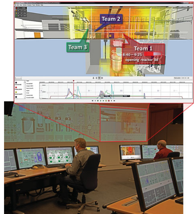
Figure 10. Monitoring of work progress from a control room of a nuclear installation supported by 3D simulation.
