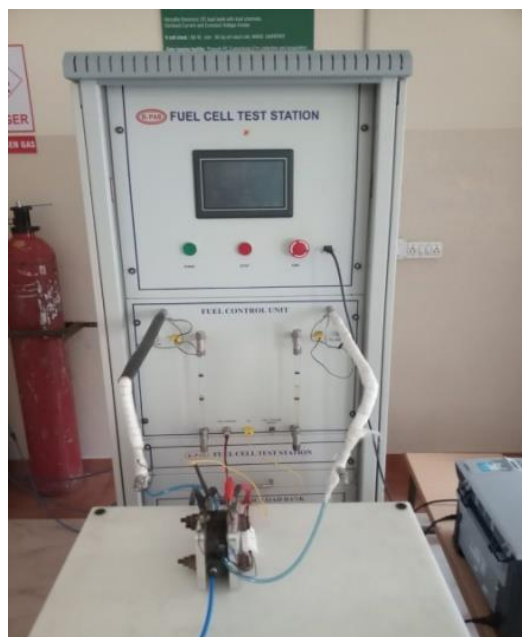
Figure 4. K-PAS fuel cell test station.
