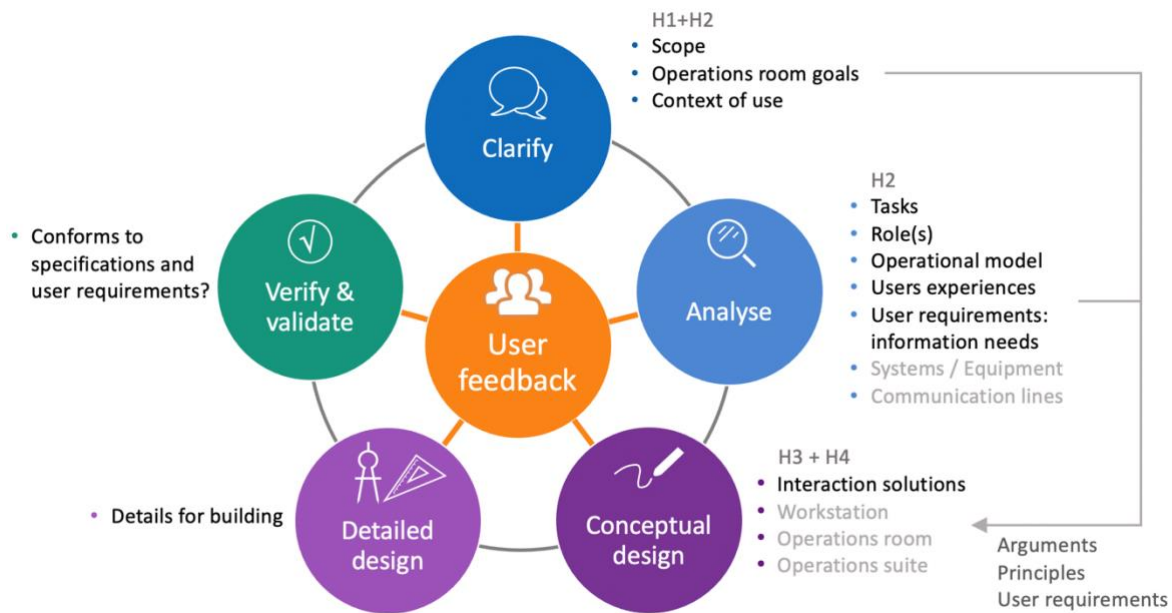
Figure 3. User-centred and iterative process for design and evaluation, and description of which phase the different LOAS work packages deals with
