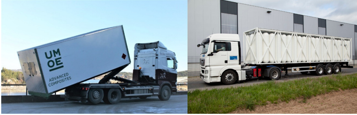
Figure 4 Transport solution of hydrogen by truck in a 20- and 40-foot hydrogen transport module [18, 19]
