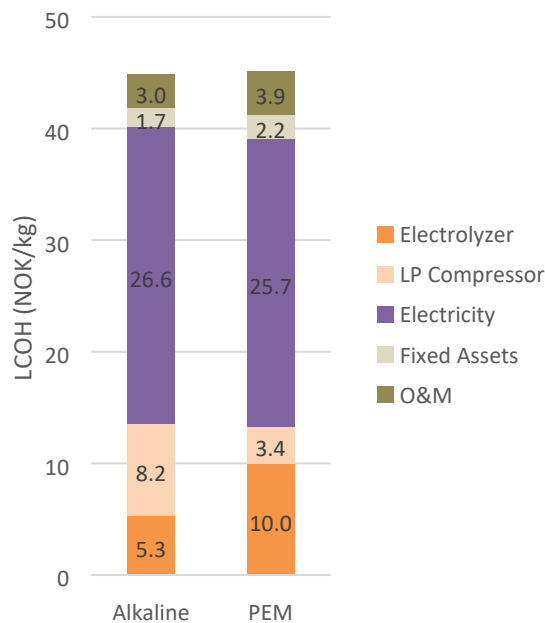
Figure 10: Levelized cost of hydrogen produced by water electrolysis and mechanical compression and supplied at 300 bar; calculations based on alkaline and PEM technologies with delivery pressures of 5 and 30 bar, respectively..
