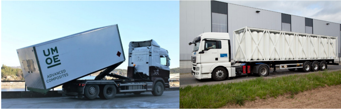
Figure B-1: Two transport solutions of hydrogen by truck in 20ft and 40ft containers/semitrailers 4,5
