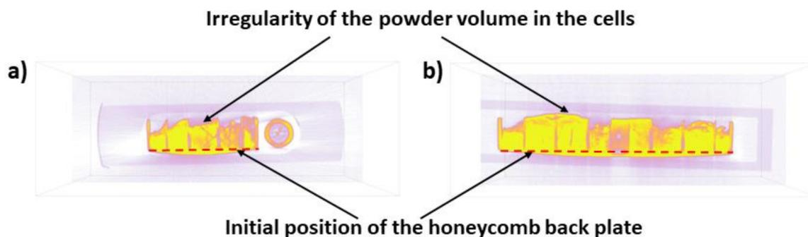
Fig. 10. Deformation of the honeycomb back plate after the  $\text{NH}_3$  absorption process (a) XY-plane, slice  $z = 394$  and (b) YZ-plane, slice  $x = 310$ . The red dashed lines represent the position of the back plate before the absorption process.
