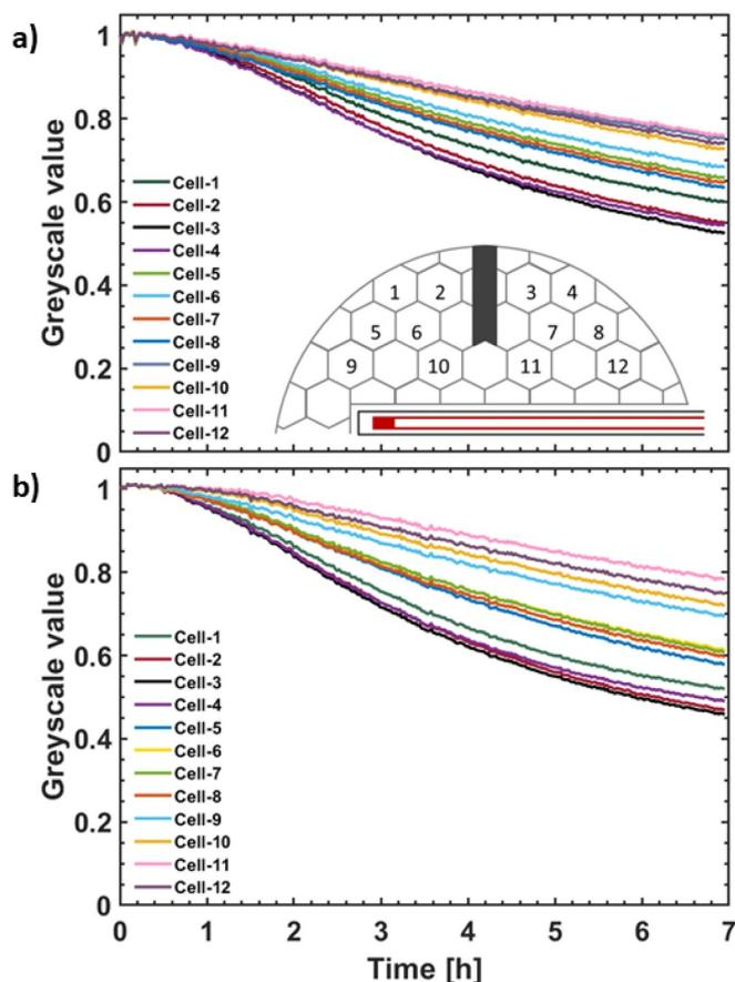
Fig. 5. The change in transmission  $I(\lambda)$  through the powder during (a) absorption-2 and (b) absorption-3. The schematic view of the honeycomb with selected and numbered cells is included in graph a.
