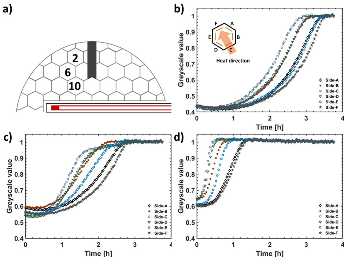
Fig. 8. The change of transmission  $I(\lambda)$  integrated along the selected volumes of the powder during desorption process at 100 °C (a) a schematic view of the honeycomb with the selected cells and the changes in transmission  $I(\lambda)$  along the lines drawn in cell-2 (b), cell-6 (c) and cell-10 (d). The heat direction is shown in the graph and is approximately the same in all three cases (b).
