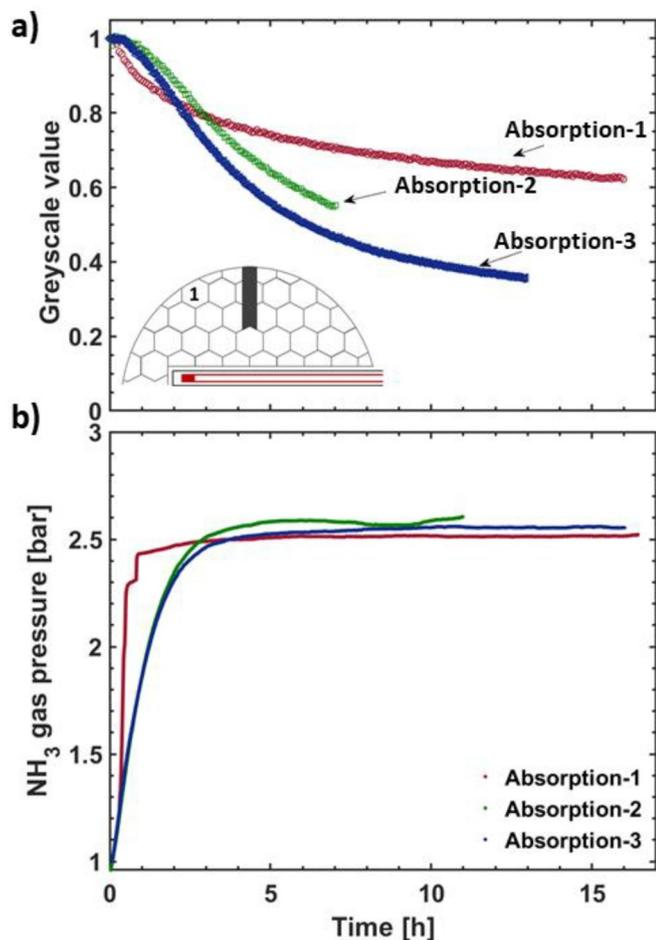
Fig. 4.  $\text{NH}_3$  gas absorption in  $\text{SrCl}_2$  contained in the THS reactor. (a) the change in transmission  $I(\lambda)$  in the cell-1 and (b)  $\text{NH}_3$  gas pressure during the absorption processes.
