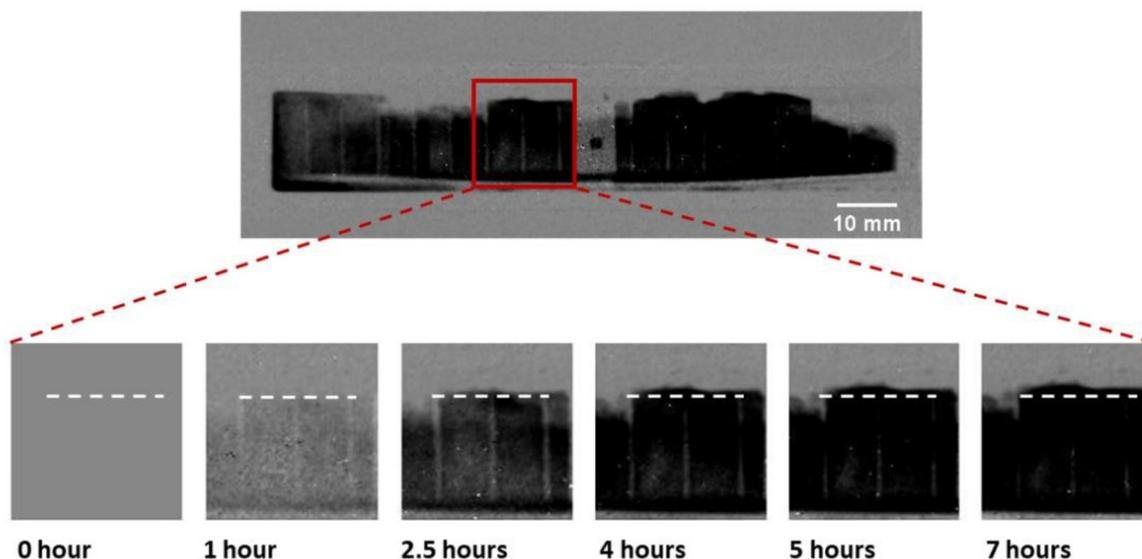
Fig. 6. Series of images showing the expansion of the salt during the  $\text{NH}_3$  absorption process with time in selected area of the honeycomb. The white dashed line shows the initial height of the powder. (Full-size image above the series was acquired at the 4th hour of absorption-4).
