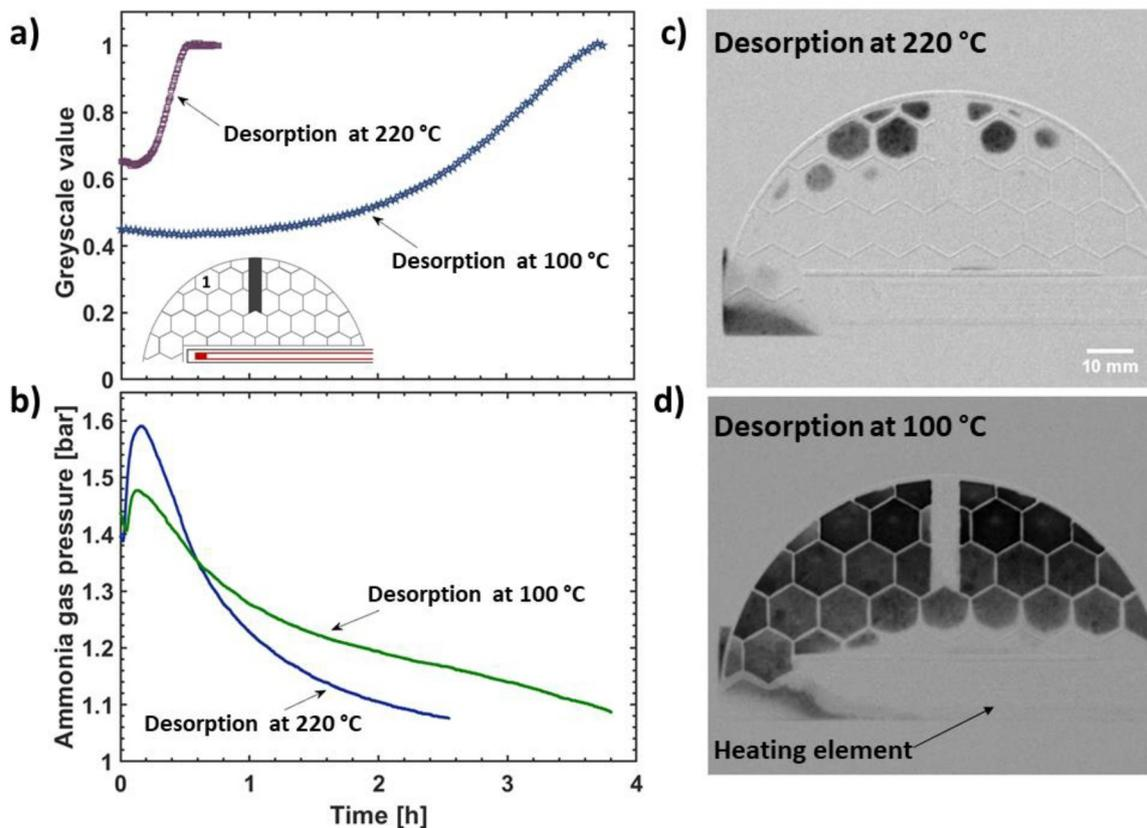
Fig. 7. The desorption processes of  $\text{SrCl}_2(\text{NH}_3)_8$  at 220 °C and 100 °C: (a) changes of the transmission  $I(\lambda)$  and (b) corresponding pressure profile. Transmission images obtained after 20 min of  $\text{NH}_3$  desorption processes performed at (c) 220 °C and (d) 100 °C.
