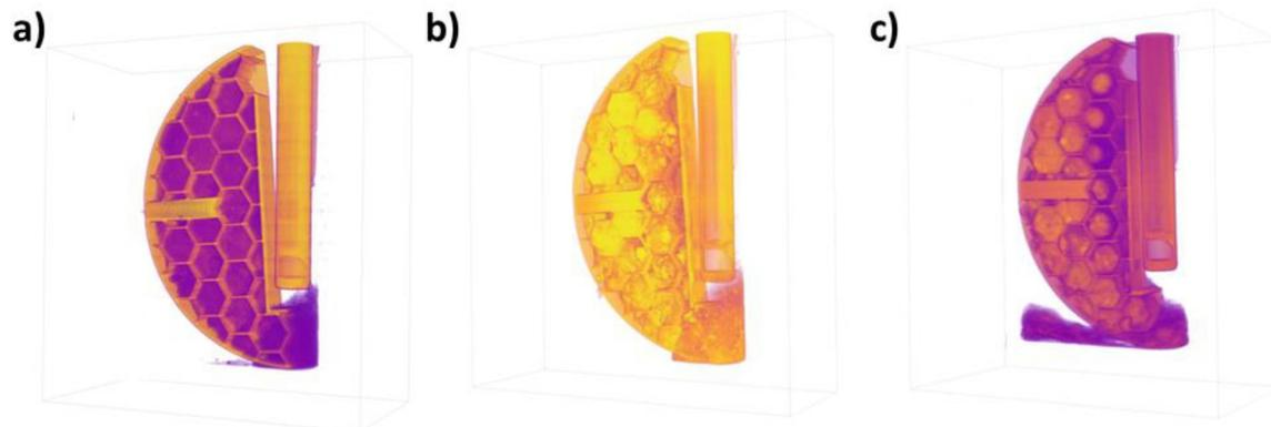
Fig. 9. 3D visualization of the honeycomb created with Tomviz software (a) fully desorbed  $\text{SrCl}_2$  salt, (b)  $\text{Sr}(\text{NH}_3)_8\text{Cl}_2$  and (c) the salt with partially desorbed  $\text{NH}_3$ . The colors of the different states are arbitrary and represented by the transmission through the absorbed  $\text{NH}_3$  intensities.
