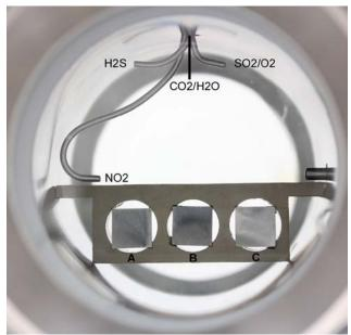
FIGURE 2. Photo of the inside of the autoclave with separate injection lines for the different impurities and holder with corrosion coupons. Coupon A was N10276 (nickel-alloy), coupon B was S355MC (carbon steel), and coupon C was S32205 (duplex stainless steel).
