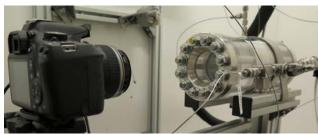
FIGURE 1. Photo showing the camera and the transparent autoclave with dosing and analyzing lines connected.
