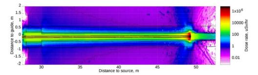
Fig. 3. Dose rate distribution in the shielding around BIFROST guide, cut by horizontal plane at guide height.
