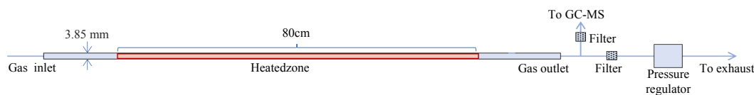
Fig. 1. Sketch of the horizontal tubular free-space-reactor in which we conduct our monosilane pyrolysis experiments.
