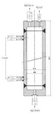
Figure 7: Water/hydrogen separator vessel (Ta-03), designed for pressures up to 350 bar.
