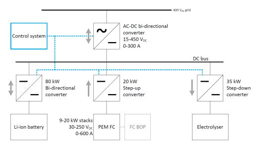
Figure 3: Electrical system and power converters of the systems laboratory at IFE.
