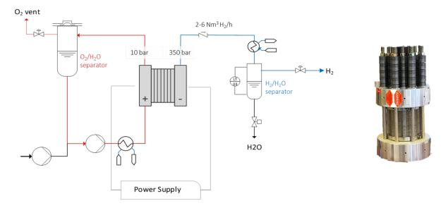
Figure 1: Sketch of WE system test rig (left) and prototype PEMWE stack operable at differential pressures up to 350 bar (right).
