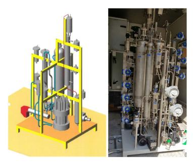
Figure 2: Mechanical design and photo of the PEMWE system test rig.
