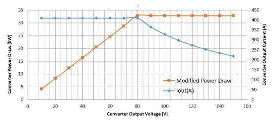
Figure 4: Output characteristics of DC/DC converter for water electrolyser system.
