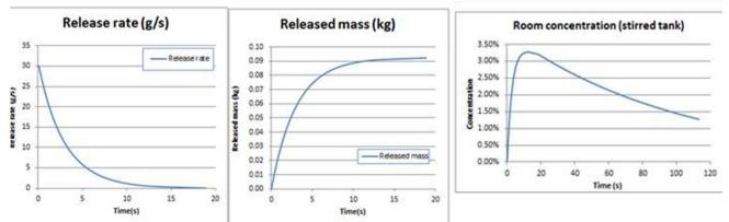
**Figure 8:** Transients associated with a severe hydrogen release (1.9 mm hole in 6 L hydrogen tank at 200 bar) in the PEMWE system container at IFE.
