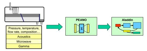
Figure 7. PEANO and ALADDIN processing data from a separator.
