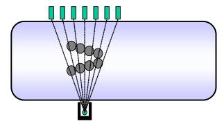
Figure 6. Gamma source and array of detectors for cyclone presence detection (separator seen from above).
