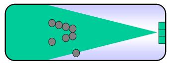
Figure 5. Microwave transmitter and detector array (separator seen from above, with one out-of-place inlet cyclone).
