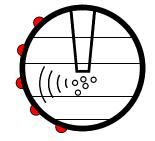
Figure 4. Acoustic sensors placed on outer separator wall.
