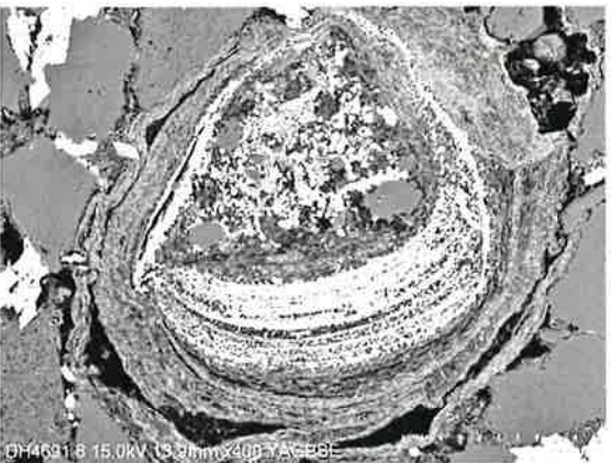
Various oolite textures: circular orientation of pale Ca-phosphate and grey chlorite. Right: tiny quartz included in center.
