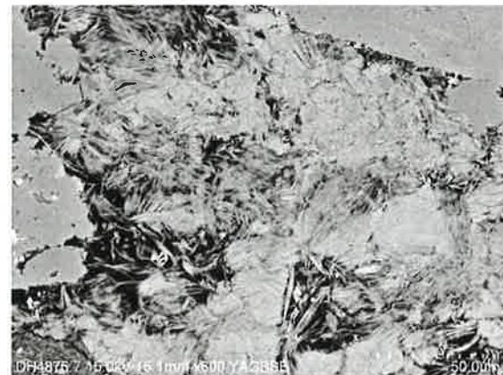
Left: Clays/ductile clasts: Chlorite in center (pale), surrounded by mica/illite (grey), quartz (arrows) Right: Pore fill with illite/mica, possibly including some kaoline.
