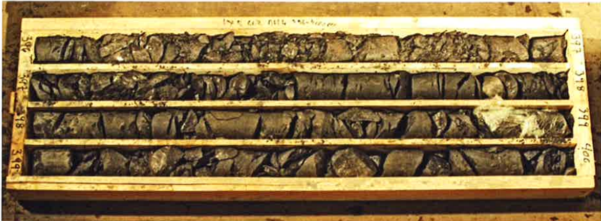
Figure 7 Core photo of the fractured zone in Dh4, 398-400m.
