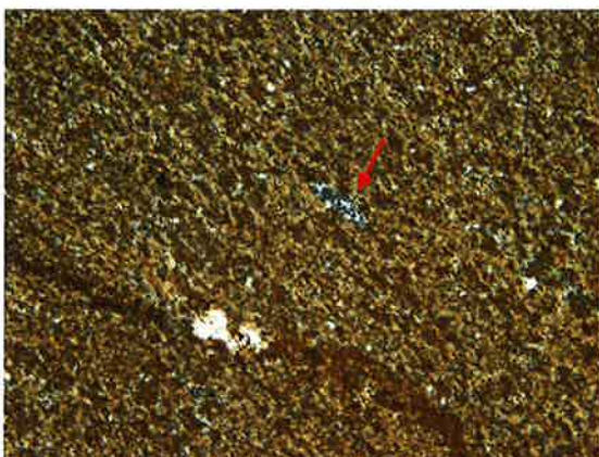
Carbonate cement (pale), microcrystalline quartz (arrow)
