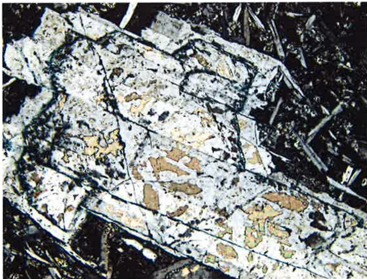
Alteration of plagioclase phenocryst to calcite
