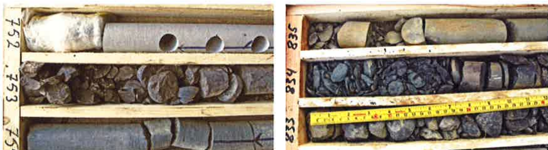
Figure 12 Crushed zones at ≈ 753m in Dh4(left), and 833.8m in Dh2 (right)
