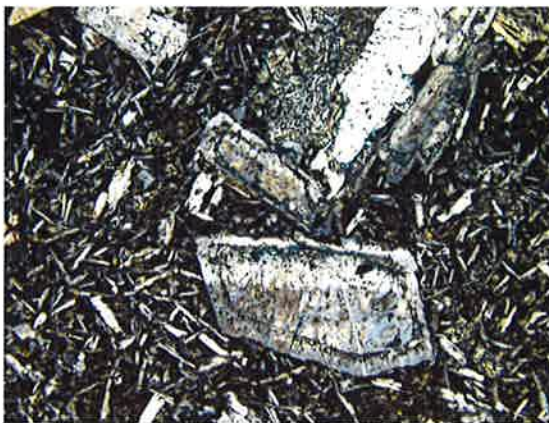
Zoned plagioclase phenocrysts.. Dark groundmass with tiny pyrites/oxides, numerous unoriented plagioclase laths.
