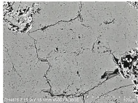
Left: Fractured quartz grains. Chlorite (Chl), alkali feldspar above. Right: compaction
