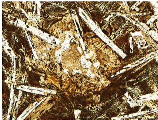
Closer view of groundmass, pseudomorph of olivine/pyroxene in center.
