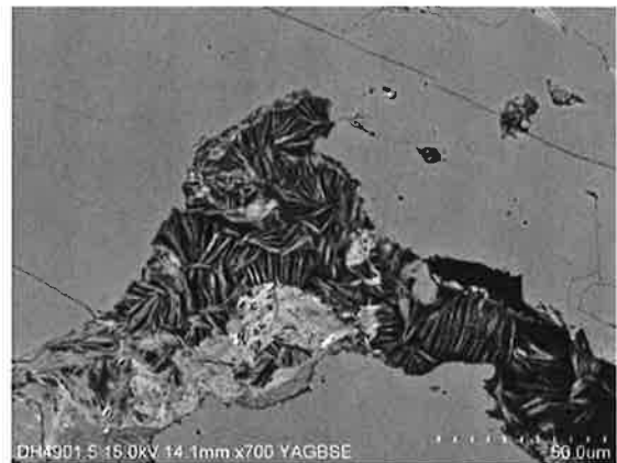
Left: Clay pore fill: in center illitic clay, down right a mix of illite and chlorite (pale) Right: Clay mix of illite, chlorite and muscovite remnants
