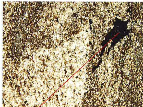
Textural overview, inhomogeneous bedding, black organics with pyrite x4 lln
