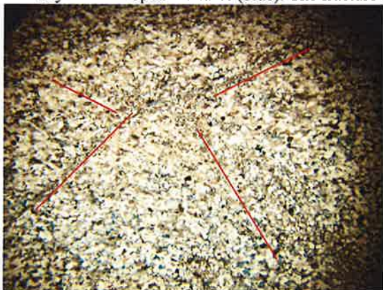
Overview showing outlined directions of possible fractures often very poorly defined, sometimes open and sometimes not. x1.5 lln
