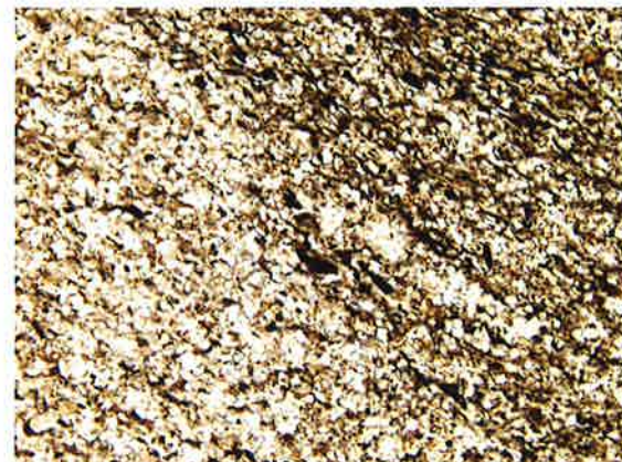
Closer view of texture, local carbonate cement (arrow), black organics, oriented mica laths x10 xn
