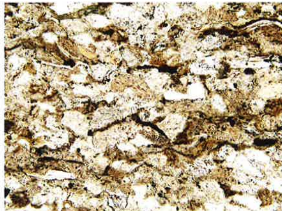
Closer view of "clay clasts", the relation to mica alteration is often obvious
