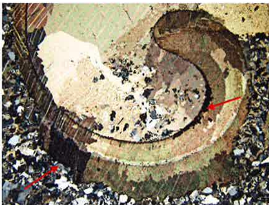
Calcite bioclast, pyrite (arrows), coarse calcite in center x4 xn
