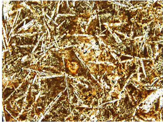
Closer view of groundmass, pseudomorph of olivine/pyroxene in center.
