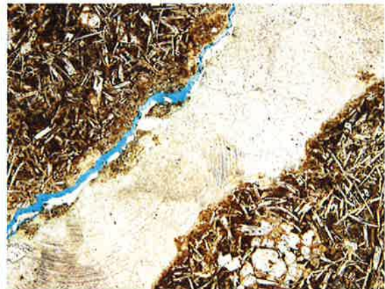
Calcite cemented fracture, smnall open fracture is probably due to preparation x4 xn
