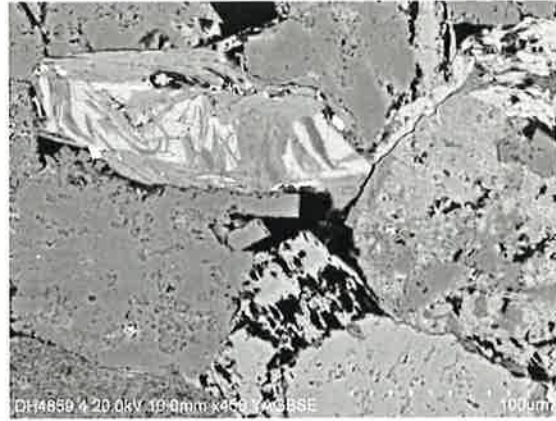
Left: In center microcrystalline quartz (chert) appearing as cement without obvious relation to surrounding quartz grains, the straight border of the quartz grain above suggests also authigenic growth. K-feldspar is partially dissolved (arrow), dense chlorite is seen upper left (detrital?) Right: Common pore view; dissolving K-feldspar and alkali feldspar (right), altering micas with muscovite, chlorite and some kaoline, authigenic albite (center). Poorly connected pore volumes.
