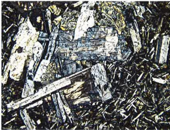
Typical dolerite texture, plagioclase laths x4 xn
