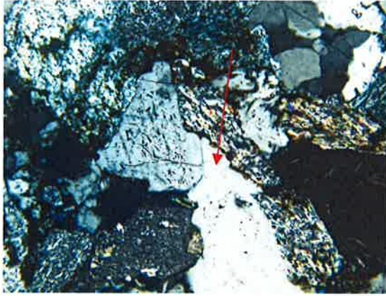
Feldspar overgrowth > quartz cement (arrow). Altered grains and fragments x20 xn
