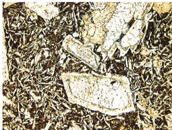
Zoned plagioclase phenocrysts.. Dark groundmass with tiny pyrites/oxides, numerous unoriented plagioclase laths.
