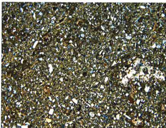
Textural overview, carbonate (altered fossil?) right (arrow). Dark greenish brown matrix x4 ln x4 xn
