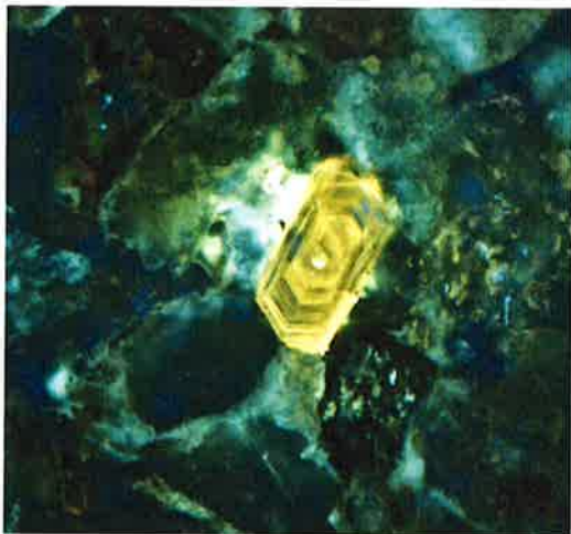
Zoned zircon seen in UV mode- length of crystal : 0.1mm
