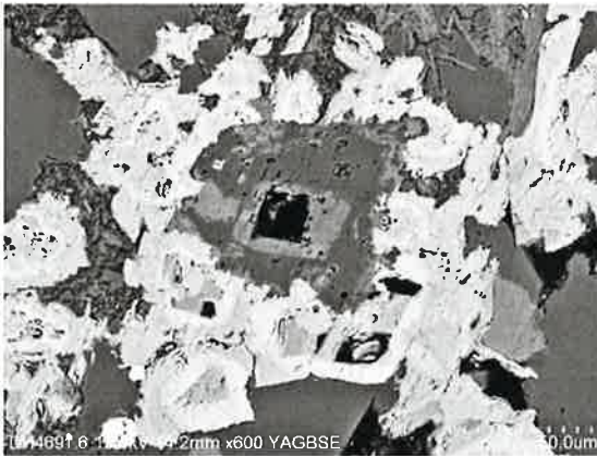
Left: Detail of complex Fe-Mg carbonate Right: Chloritic clay, quartz and Ti-oxide (small, pale grain) in pore, corroding carbonate cement.
