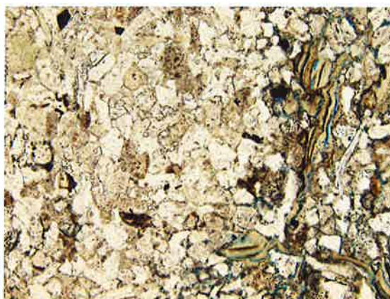
Closer view, local carbonate cement, blurred grain boundaries, wavy compacted mica
