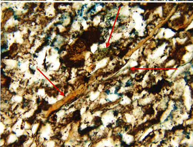
Close view, arrows show micas (biotite, muscovite, chlorite)
