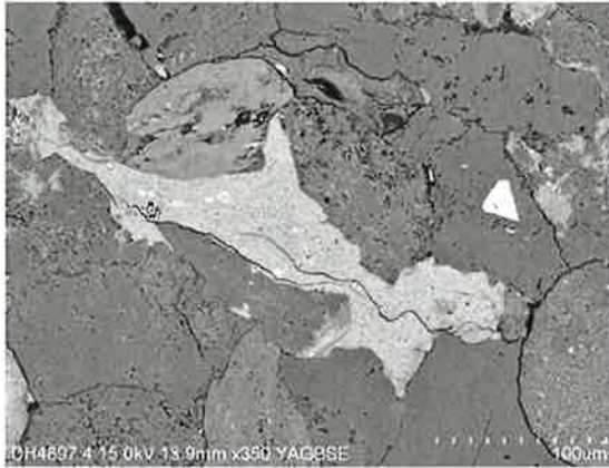
Left: Compacted texture, chlorite±illite in center. The altered circular grain down right shows a mix of K-feldspar and illite ± kaolinite. Right: Similar compacted texture, K-feldspar in center (pale).
