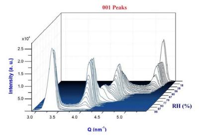
Figure: XRD pattern of Li-Fh as function of relative humidity (RH) and the scattering vector (Q).
