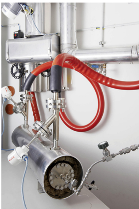
Fig. 11 – The sodium alanate-based hydrogen storage tank developed during the NESSHY project showing the attachments to the testing rig.
