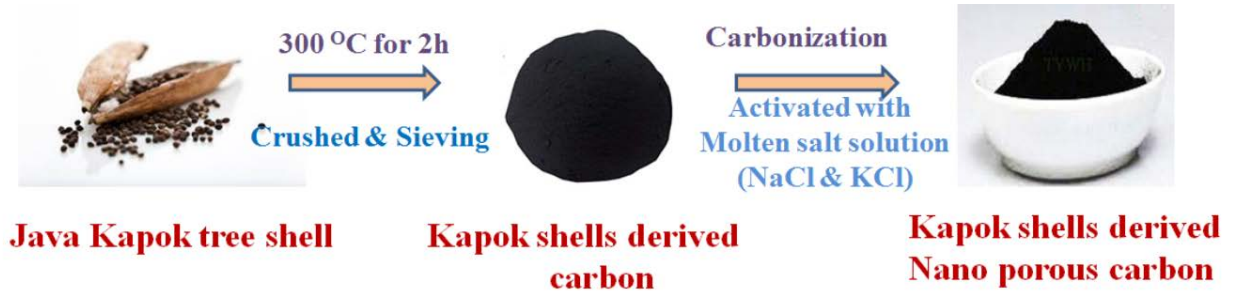
Figure- Schematic illustration kapok shell derived nanoporous carbon formation.
