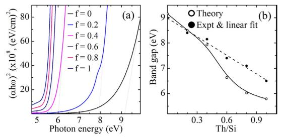
Fig 5. Tauc plot for  $SiO_2$  and  $ThO_2$  obtained by first-principles calculations and for  $SiO_2/ThO_2$  composites obtained by Bruggeman effective medium approximation (a); dependence of the band gap on fill factor Th/Si (open circles and solid line) calculated by effective mass theory and (filed circles and dashes) established experimentally (b).
