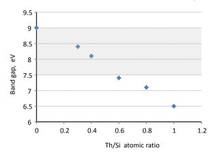
Fig.4 Bandgap depending on local concentration of thorium atoms acording the results of chemical composition analysis of the surface with XPS and REELS methods
