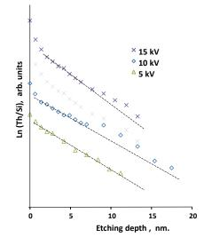
Fig.2 Depth profile with Ar etching for samples ThSiO<sub>X</sub>/SiO<sub>2</sub>/Si formed after Th implantation during PLD deposition under various high voltage
