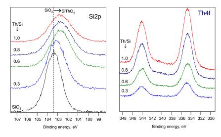
Fig.1 XPS spectra of Si2p and Th4f lines for sample with different Th/Si atomic ratio in near-surface SiTh<sub>x</sub>O<sub>y</sub> region formed after Th implantation during PLD deposition under high voltage 15 kV
