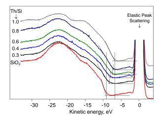
Fig.3 Reflection Electron Energy-loss Spectra with energy 1000 eV scattered on surface of Si/SiO2 samples for different Th/Si atomic ratio in near-surface ThSi<sub>x</sub>O<sub>y</sub> region formed after Th implantation during PLD deposition under high voltage 15 kV
