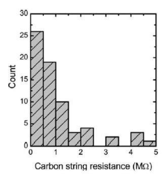
FIG. 8. Resistance for 68 conducting CB strings on glass substrate.
