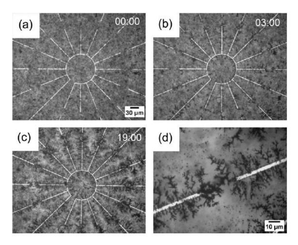
FIG. 6. Electric field alignment on conducting silicon substrate covered by SiO<sub>2</sub> layer.
