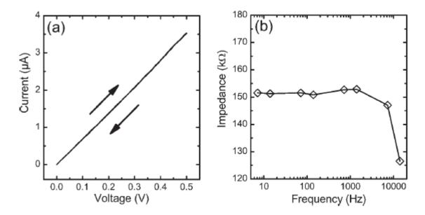
FIG. 7. (a) IV-loop and (b) impedance for one aligned CB string on glass substrate.
