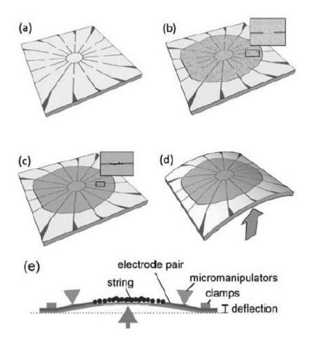
**FIG. 2.** Schematics of alignment procedure. (a) The electrode pattern deposited on substrate. (b) CB - oligomer mixture spread on the electrodes. (c) Aligned CB strings between electrodes after electric field treatment and polymerization of matrix. (d) Bending of silicon substrate with aligned strings. (e) Setting to measure strings individually. Not drawn to scale.
