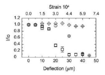
**FIG. 11.** Relative changes of current as a function of deflection for two different aligned carbon strings on silicon substrate (black squares and red circles). Also shown are corresponding data for non-aligned film with 12 vol. % carbon loading (cyan diamonds).
