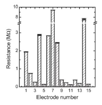
**FIG. 9.** Resistance of aligned strings on one alignment substrate with 15 simultaneously used electrode pairs, counted clockwise around the electrode configuration.
