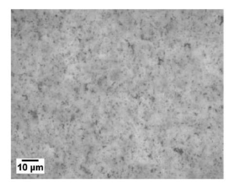
FIG. 3. Isotropic mixture of CB particles in oligomer fluid.
