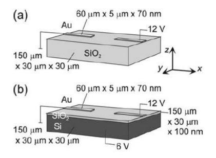
**FIG. 1.** Schematics of alignment electrodes used in simulations. The electrode patterns on glass (a) or silicon substrate covered by insulating  $SiO_2$  layer (b). Not drawn to scale.
