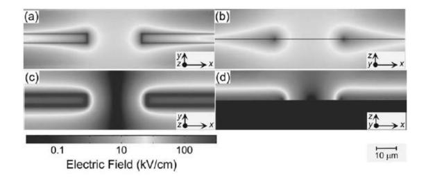
**FIG. 4.** (a-b) Simulated magnitude of the electric field on glass substrate and (c,d) on conducting silicon substrate covered by insulating  $SiO_2$  layer. The distributions (a,c) are along the surface normal, cut at 140 nm above the substrates and thus 70 nm above the electrodes. The distributions (b,d) are shown perpendicular to the electrode tips and the surface normal.
