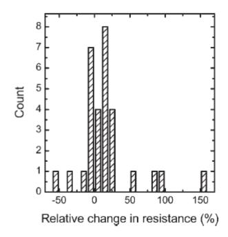
**FIG. 10.** Relative change in resistance in 30 CB strings between measurements immediately after curing and after three weeks aging period.
